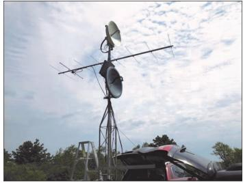
dish and transverter. It uses a thrust collar on the top to relieve strain on the rotor. We leveled and bolted it to an existing pipe. I then set up the station inside a very nice room with TV and internet. Really roughing it! A test QSO was made with Ed, W3EKT.
