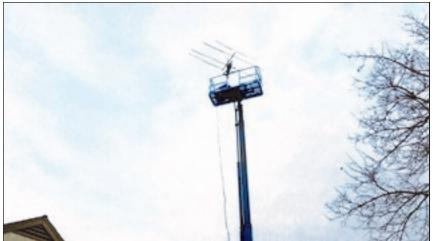
this technology to his station. Tower erection getting tougher? He came up with the innovative idea of using a bucket truck(s) in lieu of towers to quickly raise the antennas in position. His good friend and member, Bill, K1DY was quick to support Stan with all of the designs.
